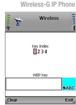
Figure 4-24: Enter WEP Key (for Secured Network)
